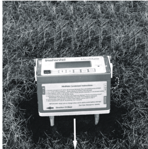
Figure 3-2 Installing the MiniMate using the Ground Spikes.
