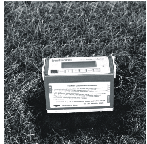
Figure 3-3 Final Installation with Ground Spikes Pushed Fully into the Ground.
