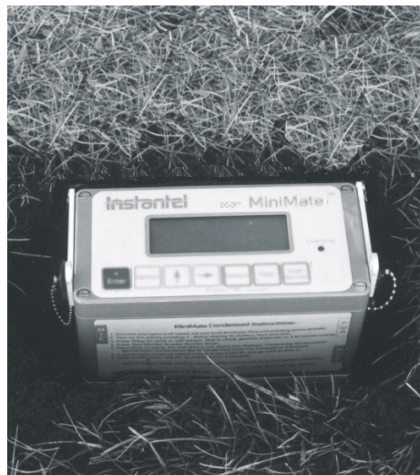
Figure 3-4 Burying the MiniMate. Protect the Monitor with a Plastic Bag.
